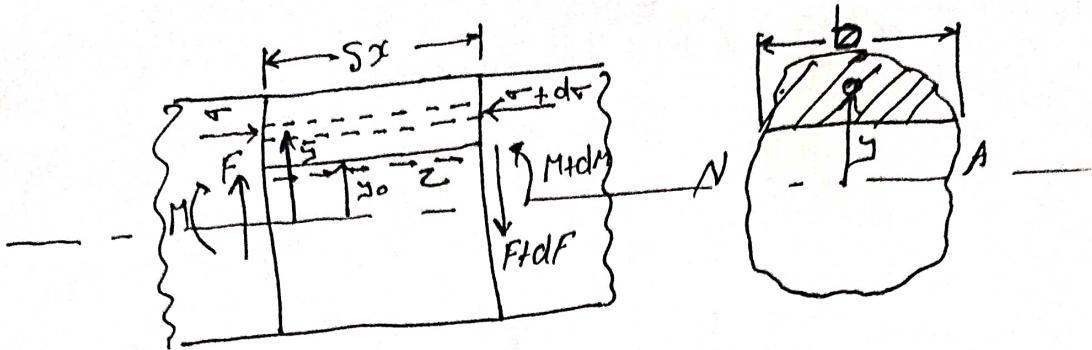
about, the shearing force & bending moments being  $F$ ,  $F+sf$  &  $M$ ,  $M+dm$  respectively.
