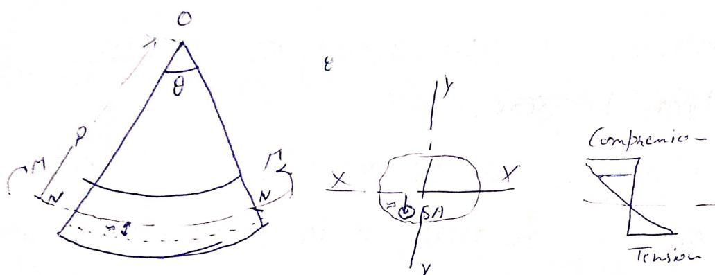
From fig. it is clear that end sections remain plane & that for initially straight beam the inside or concave edge will be in compression & the outside or convex edge will be in tension. There will be an intermediate surface at which shear is zero ("neutral" surface); the neutral surface cuts any cross-section in the neutral axis.
