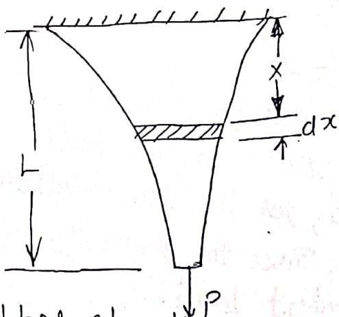
where  $A$  is area of cross-section of bar at section  $x$
