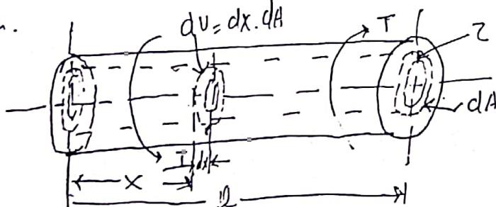
Consider a section of the shaft at a distance  $x$  from left end. Let  $\tau$  be the shear stress acting on the elementary area  $dA$  at a distance  $z$  from the centre. Then the strain energy stored in the elementary strip due to torsion, known as the torsional strain energy,
