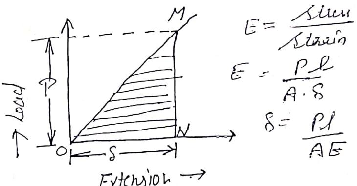
Work done in straining the bar = Area of Load extension curve
